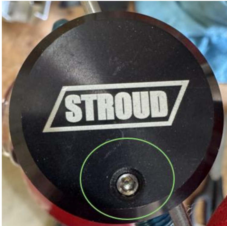
Figure 2: Set Screw Location
