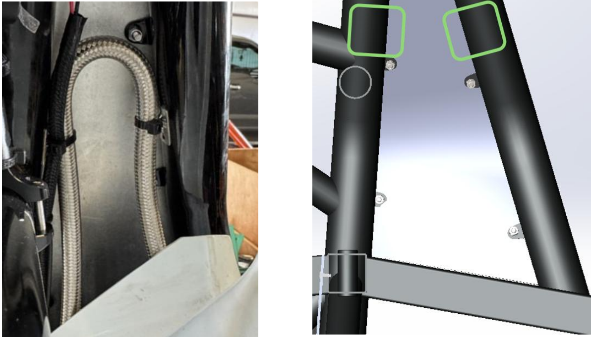
Figure 13: Vent Line Location
